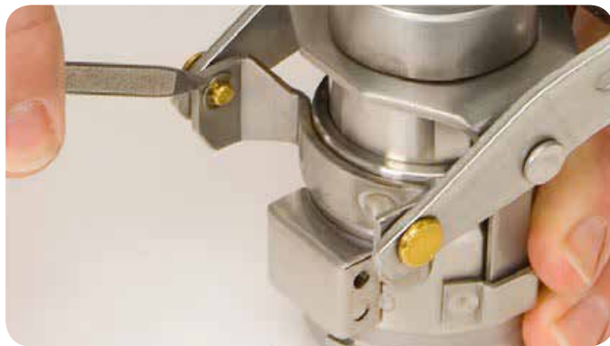
3. Disassemble coupler by removing c-clips and clevis pins in order to replace o-ring seal.
