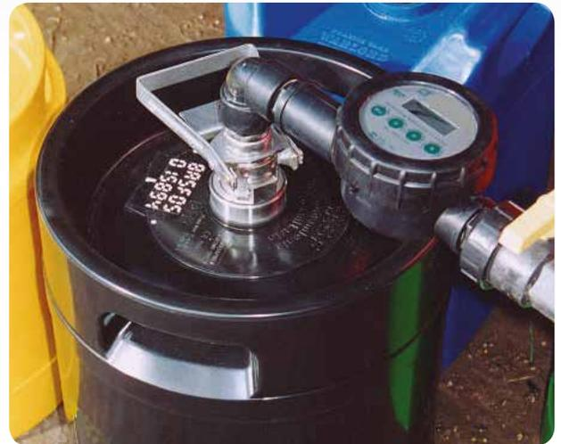
*The Farmtainer with Micro Matic Drum Valve, the dry-break Coupler and the flowmeter to measure the exact dosage required for optimum effect.*
