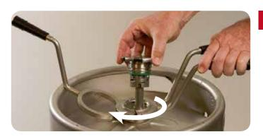
7. With your free hand pull up while turning clockwise on extractor valve until it is free from the container.
