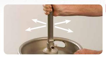
by using the Verification Tool #741-043. Place the service tool on the extractor valve flange and rotate it 1/6 of a turn clockwise.
