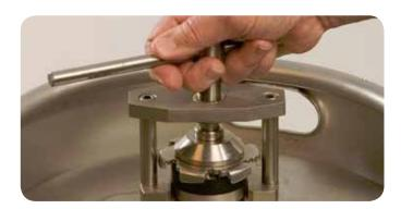
7. Place Spindle Tool #740-076 over the extractor valve as shown.
