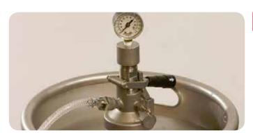
Option - Pressurized Leak Testing by using the MAV Pressure Test Head #748-XXX.
