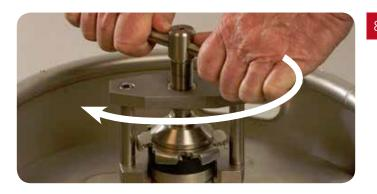
Lock the extractor valve securely in place by turning the spindle handle clockwise until no more clicks are heard.
