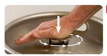
6. IMPORTANT: It is necessary to seat the extractor valve properly in the neck prior to step 7.
