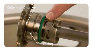
Inspect extractor valve O-ring and Retaining Ring for damage.
