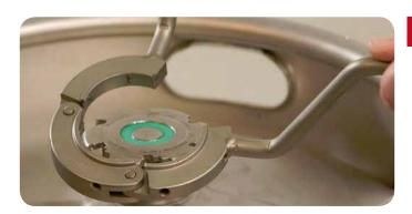
Place the Valve Releasing Tool #740-078 so that the six pins fit into the six corresponding holes in the container under the extractor valve flange.
