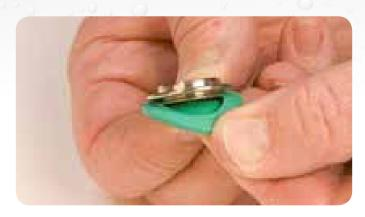
Install new dry break seal on insert.
