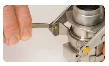
Disassemble coupler by removing c-clips and clevis pins in order to replace o-ring seal.
