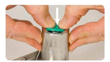
6. Press the new dry break seal assembly firmly into the probe until the dry break seal locks into place.
