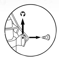
Install clevis pins and c-clips as shown.
