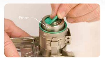
Remove dry break seal from probe and discard.
