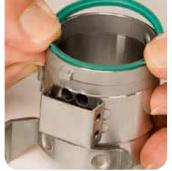
Turn coupler body upside down. Clean main seal groove. Install new main seal.
