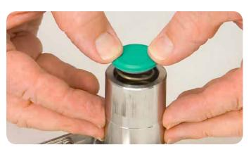
Install spring by placing the largest end of spring into the probe and wiggle in a clockwise direction while pressing down firmly.
