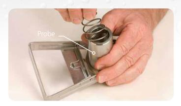
Install spring by placing the largest end of spring into the probe and wiggle in a clockwise direction while pressing down firmly.
