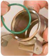
7. Remove O-ring seal from coupler body and discard
