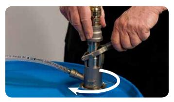
Rotate Heavy Duty Coupler clockwise 1/3 turn until it stops.
