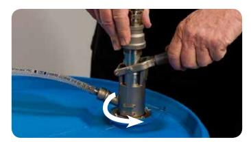
2. Rotate coupler counter clockwise 1/3 turn until it stops.
