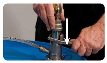
Engage the coupler by pushing down on the handle.
