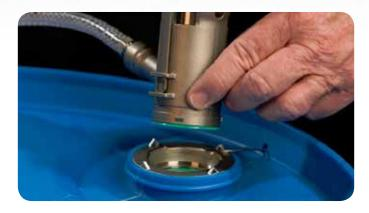
2. Align Heavy Duty Coupler pins with corresponding slots in RSV/DV valve.
