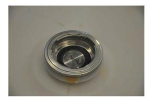
Ensure the valve recess and face is free of dirt and grit.
