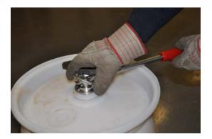
10. When the clinch ring is removed it will have sharp edges, handle it with care using leather gloves and place it in a scrap bin.
