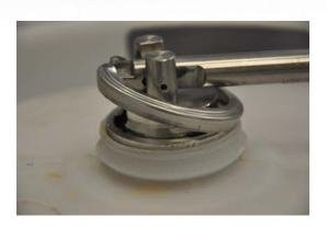
g. In some cases it might be necessary to remove the tool from the valve and then re insert it but starting from the next bayonet slot and work on the clinch ring in a different position (120 degrees for a 3 pin and 90 degrees for a 4 pin) this will allow the clinch ring to be released from the container neck.
