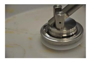
7. When the first movement has lifted the edge of the clinch ring release the pressure on the red handle and reposition the tip further into the space that has been made and push the red handle forwards and when the chisel tip is fully inserted gradually press the red handle down to lift the clinch ring further.
