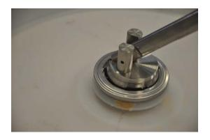
4. Rotate the tool clockwise to engage the bayonet pins and until the chisel tip can access the inner edge of the clinch ring – DO NOT rotate the tool so far that the valve is being rotated as this will damage the tool.
