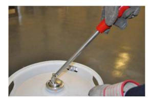
Hold the red handle of the clinchring removal tool in one hand and guide the disc and bayonet features into the face of the valve with the other.
