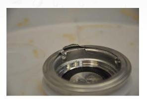
Move the red handle down and forward and carefully lever up the inner edge to stretch the clinch ring up from the inner edge towards the outer edge.
