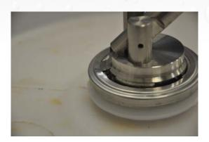
5. Raise the red handle and manoeuvre the chisel tip corner into the position shown between the inner edge of the clinch ring and the top of the valve.
