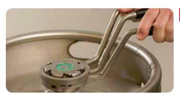
Turn Lifting Tool #740-077 handle clockwise until the extractor valve moves up.
