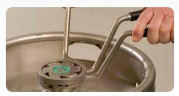
Place the Lifting Tool #740-077 on top of the Valve Releasing Tool.
