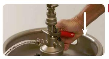
Push down on the handle to engage the Fill Head. If engaged correctly, the handle will lock into position.
