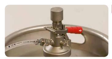
Degas container with MAV Degas Head #748-XXX.
