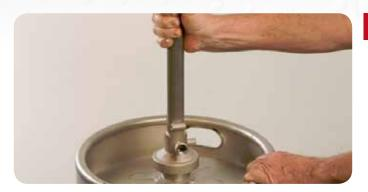
9. Verify that the extractor valve has been installed correctly by using the Verification Tool #741-043. Place the service tool on the extractor valve flange and rotate it 1/6 of a turn clockwise.
