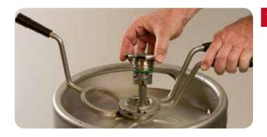
With your free hand pull up while turning clockwise on extractor valve until it is free from the container.
