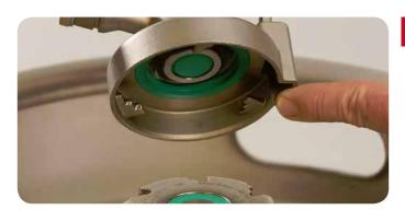
Align MAV Fill Head pins with slots in MAV Valve.
