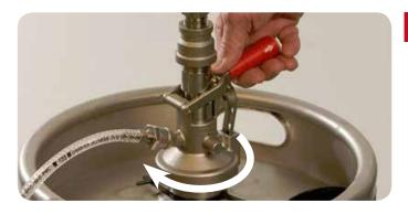
Rotate MAV Fill Head 1/6 of a turn clockwise.
