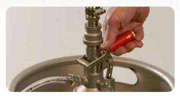
1. MAV Vapour Recovery Fill Head with filling hose and vopor recovery hose attached
