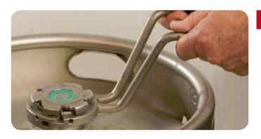
Squeeze the Valve Releasing Tool handles gently to compress the Circlip.
