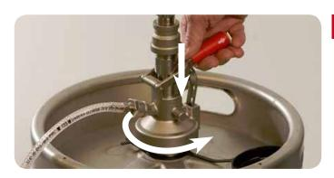
2. Rotate MAV Fill Head 1/6 of a turn counter clockwise. The Fill Head can now be moved.
