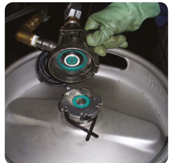
Macro Valve Fill-head: On disconnection there is no product residue on the Macro Valve and Coupler
